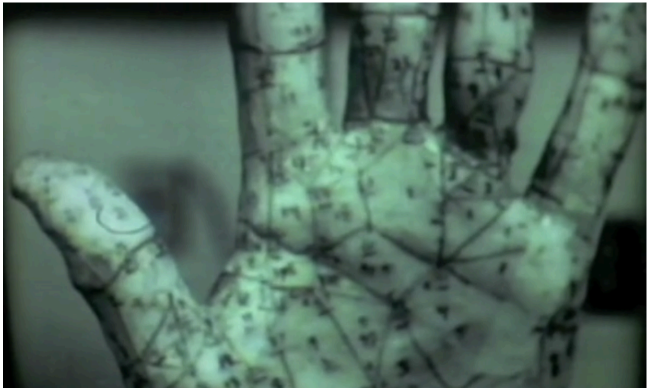
[Figure 19: Detail of a plaster mold of Edwin Catmull's hand, marked with polygons for digitization, 1971]
