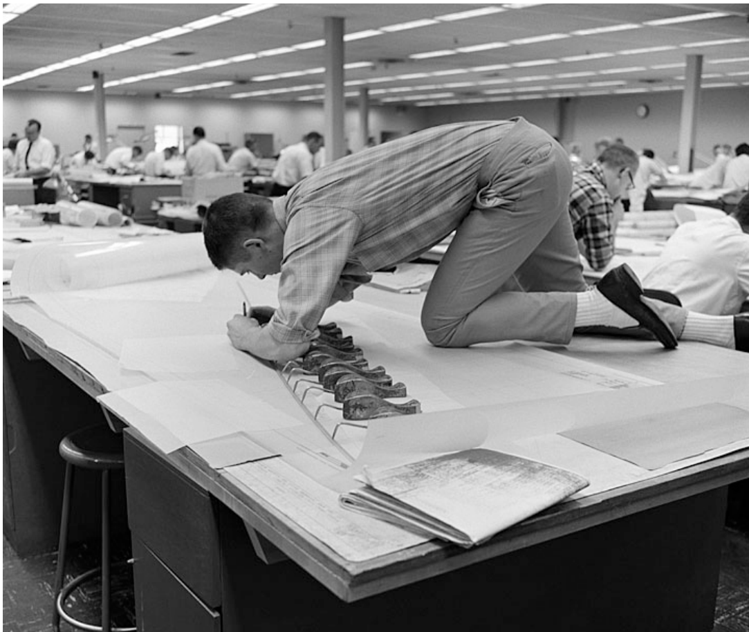
[Figure 4: A draftsman at Boeing working with spline ducks while lofting.]
